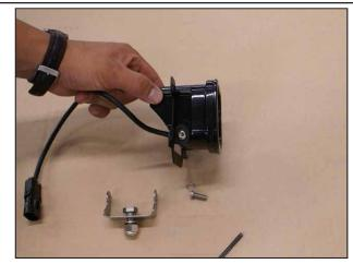
Replace Baja Designs mounting brackets with Rally Innovations brackets. Ensure that the tabs face forward.
